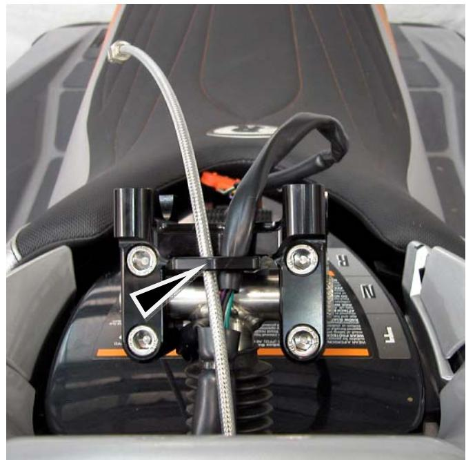
Install D.E.S.S. post into D.E.S.S. mount on back of Bar Mount. **NOTE: Do not over tighten nut.**
