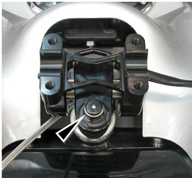
Install handlebars. **NOTE: Supplied spacers must be used for stock or 7/8" O.D. bars. Do not use spacers with 1-1/8" bars.**
