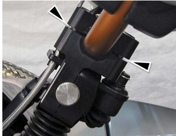
Remove top half of handlebar clamp.
