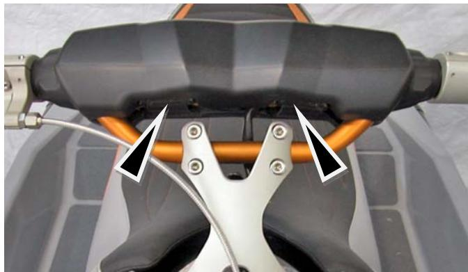
Remove throttle cable from throttle lever. Remove multi function switch housing (4 bolts). Cut and remove zip tie securing electrical wires to stock handlebars.
